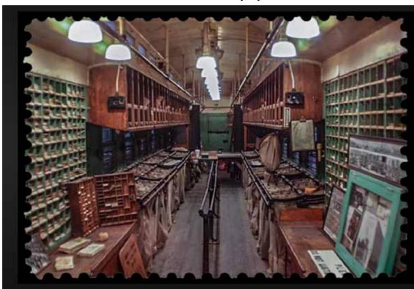
Interior of an RPO car. Priority (local) mail was sorted in front of the pigeon holes, from where it would be grabbed, wrapped with the ID of the RPO clerk who did the sorting, and bagged to be thrown off the train at the appropriate station. The iron rack running down the center supported sorting tables hung between the bars next to the large bags and the center. RPO clerks would dump the long distance bags on such a table and throw the items into the proper bags. (russeirayphotos2.com)
